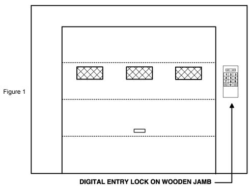
IF YOU ARE MOUNTING YOUR KEYLESS ENTRY SYSTEM TO ALUMINUM SIDING you may find it better to substitute carriage bolts for the mounting screws supplied. Bolts should be long enough to reach into the garage, and be secured with lock-washers and nuts. IF YOU ARE MOUNTING YOUR KEYLESS ENTRY SYSTEM ONTO BRICK, STONE, OR MORTAR, suitable anchors must be set into the mortar, and the fasteners screwed into these.
