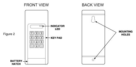
The RF Programmable Keyless Entry System has two programmable codes:
