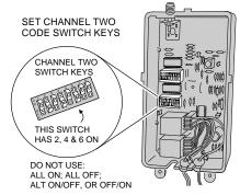
the coding switch on the transmitter and set the eight keys identical to those on the desired channel of the receiver. Be sure they match exactly. If using a two or four-channel transmitter, refer to the coding instructions included with the transmitter for proper system coding.
