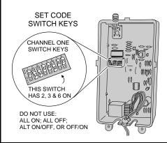
STEP 5 Connect receiver to power. Connect the red power input wire to the 24V radio power and the black wire to the common terminal on the gate operator. Alternately connect wires to a 16-24 VAC transformer.
