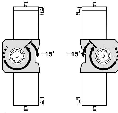
**Important:** Turn the ram pinion in the closure direction until it stops, then back by about 15° in the opposite direction. Insert the ram in the box and close the leaf. Now tighten the grub screws and raise the ram, engaging the pinion with the bushing.
