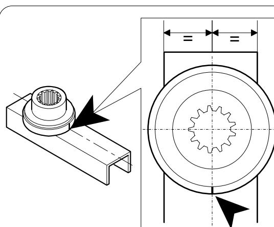
**Important:** The axis of the bushing and the axis of the guide bracket must be aligned, with the reference mark oriented towards the outer edge of the leaf as shown in the figure.
